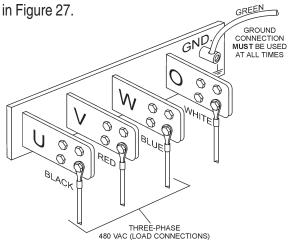
Figure 27. UVWO Terminal Lugs 3Ø-480V Connections
